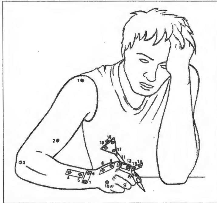
Figure 8. Configuration of 17 infrared-light emitting diodes (IREDs) allowing the accurate recording and analysis of joint angles from elbow to finger tip, as well as of the pen point and its inclination. (Schillings, Meulenbroek, and Thomassen, 1996).
