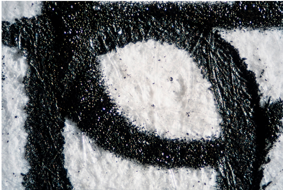
Figure 7. Carbon type over laser print. Coaxial bright field plus oblique illumination. SOX.
