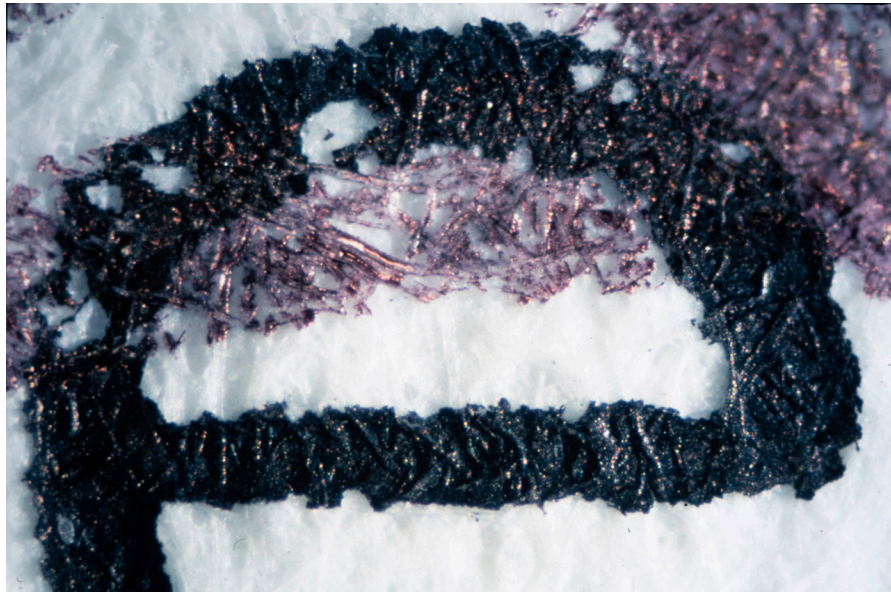
Figure 14. Ink over carbon type. CBF illumination, 40X. Sheen was clearly seen in color view; note flaking of carbon type at crossover areas.
