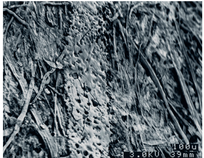
Figure 11b. Ballpoint ink over laser print. SEM with 50° tilt. 700X. At crossover. Note cracks and pooled ink.
