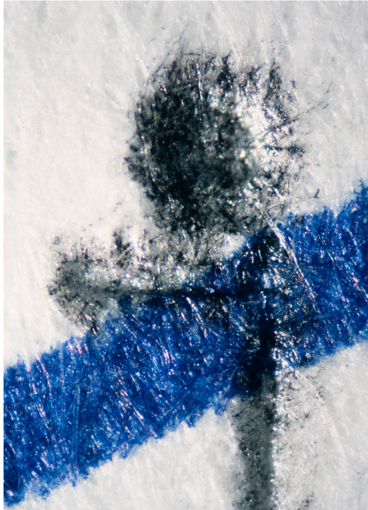
Figure 17c. Cloth typewriter over ink. Note actual continuity of ink line. In an actual case this would be judged as such, but a low level of confidence.
