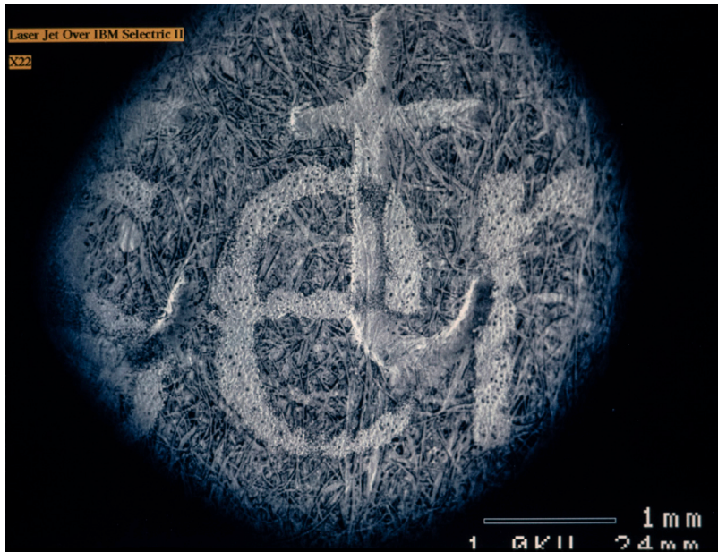
Figure 9a. Laser print over carbon type. 22X. Sequence ambiguous at this magnification, but note textural change at crossover points.
