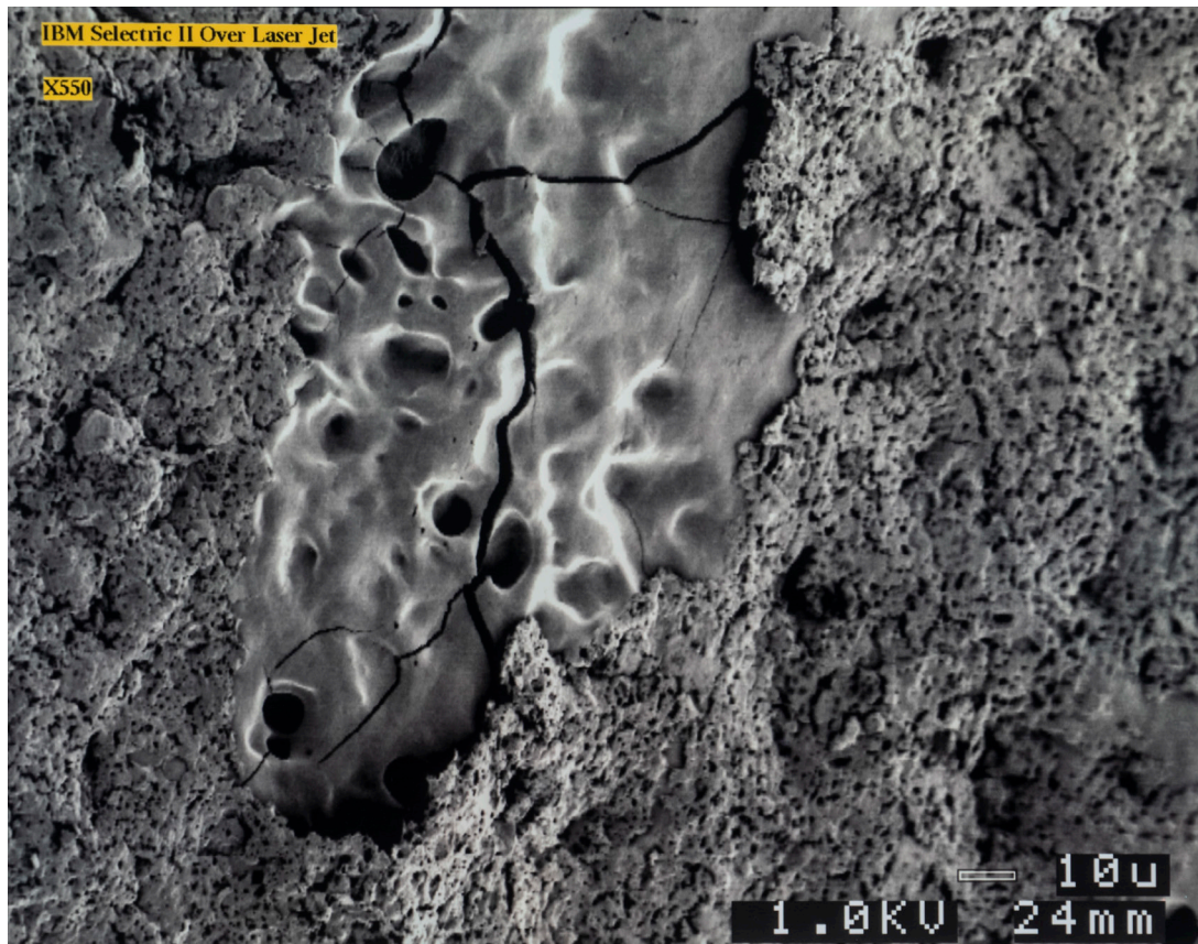
Figure 6c. Carbon type over laser print, SEM. Note continuity of carbon type in lower magnification views; high magnification view shows cracked laser print, as well as the carbon paste distinctly over the laser print.
