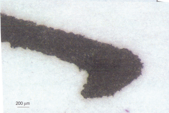
Figure 11. Pigment pooling between the paper fibers.
