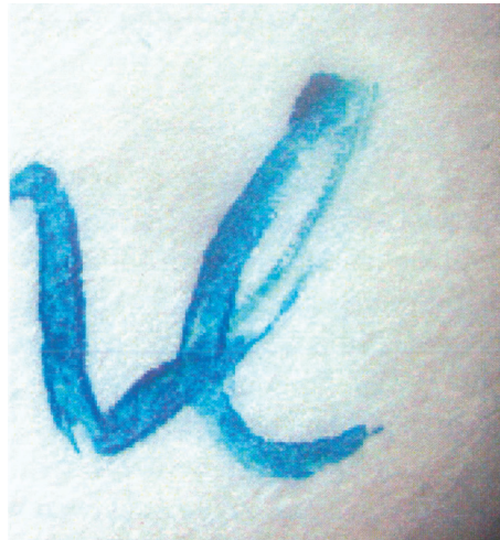
Figure 1. Irregular line quality in the writing performance of Sanford Uni Ball Signo Gel Stick, which is a common problem in gel pens as they age.
