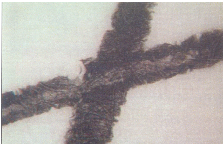
Figure 7. Light center line in Pentel Sunburst Gel K-906. The downward pressure of the writing causes the ink to flow away from the center of the nib and concentrate on the edges. Changes in pressure can produce significantly different results with the same pen.
