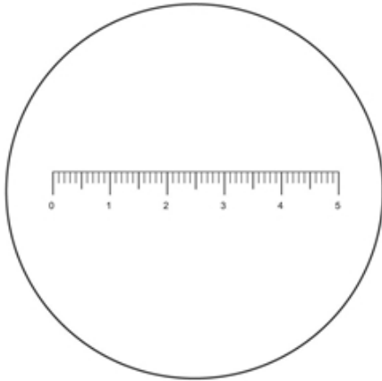
Figure 4. A reticle with this pattern is uncluttered and ideal for use. The author's reticle also has a vertical scale 90 degrees to the horizontal scale (see Figure 5).
