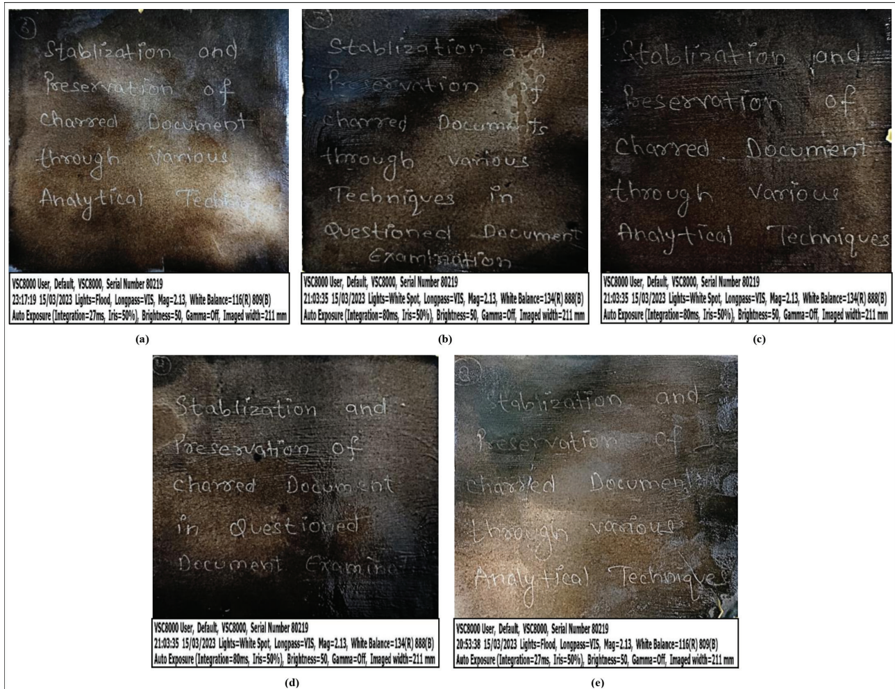
Figure 8: Visualization of coated charred documents under Video Spectral Comparator having enhanced deciphered texts.
