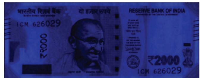
Figure 1c. A close-up photograph of the front/back side of genuine 2000-INR note under UV light at 365 nm.
