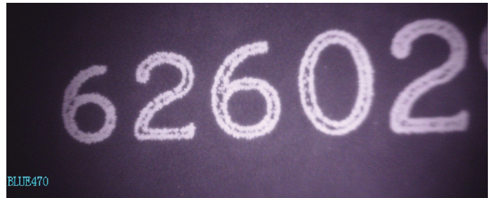
Figure 7b. IR fluorescence view of number panel in counterfeit note.
