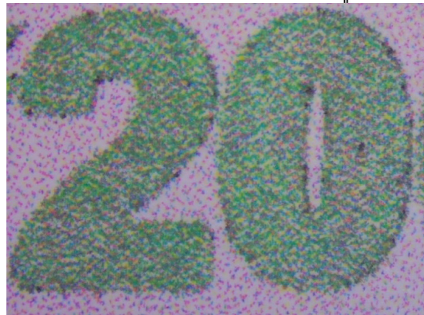
Figure 4d. A microscope image of numeral denomination shows a non-impact dot matrix pattern in a counterfeit note.
