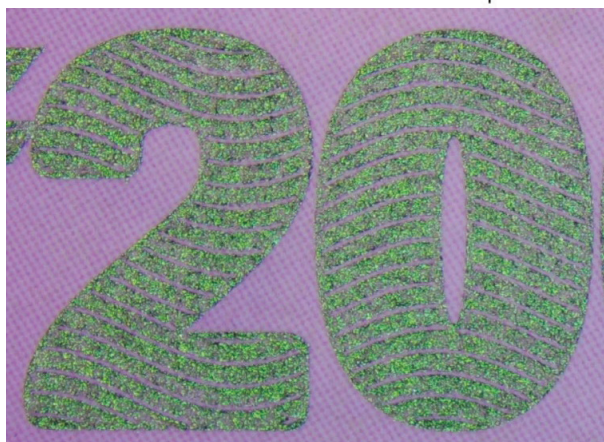
Figure 4c. A microscope image of numeral denomination (2000) shows OVI in a genuine note.
